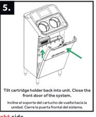
CAUTION: UPX hand hygiene solution is installed on the left. To replace SelfCleanX, follow instructions above, but install on the right side.
