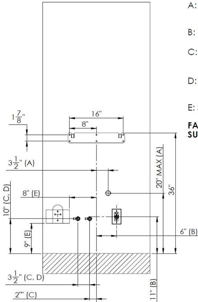
A: WALL DRAIN STUB (1½" WASTE, P-TRAP SUPPLIED BY CUSTOMER)
