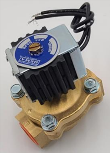
961-0900-043 1/2" NPT WATER SOLENOID VALVE, 12 VDC, EVO
