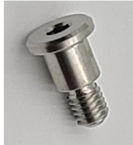
995-3154-004 10-32 X 1/4" X 1/4" SST, SHOULDER BOLT
